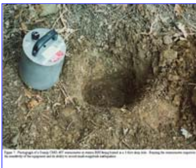
Figure 7. Photograph of a Guralp CMG-40T seismometer at station BH0 being buried in a 1-foot-deep hole. Burying the seismometer improves the sensitivity of the equipment and its ability to record small-magnitude earthquakes.
